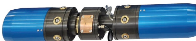
In-bore laser repair robot
