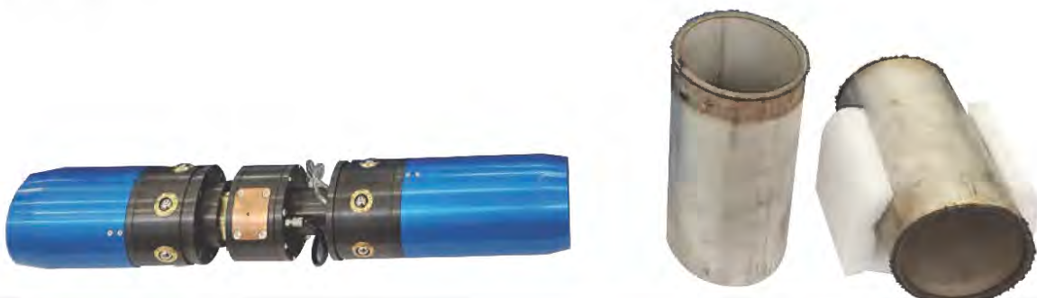
In-bore laser repair robot
