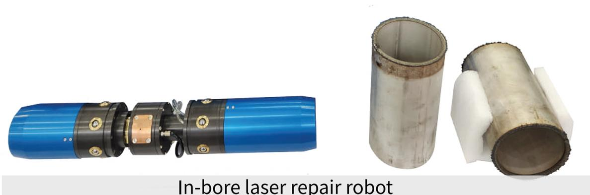
In-bore laser repair robot
